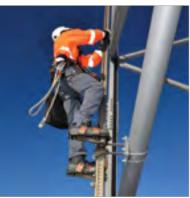
The *High Step Lift* is the world's first portable and fully automated lift platform. It is light to handle and easily clips into the HighStep Rail. The High Step Lift works using re-chargeable batteries with one full charge reaching a potential height of 1000 m with a load of 150 kg. It can be remote controlled and transport goods as well as people.
